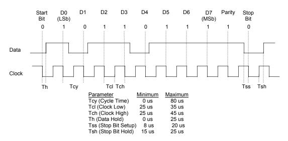
Figure 5-5. 8042-To-Keyboard Transmission of Code EDh, Timing Diagram
